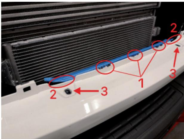
3. The M6 screw first goes through the M6 body plate, through the IVECO fastening plate, through a spacer sleeve and through another body plate and is then screwed into the existing nut pieces (3) through the plastic bumper.
